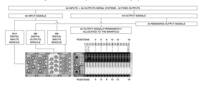
64 INPUT + 64 OUTPUT serial systems - 48 fixed OUTPUT (Ex. PROFIBUS DP and CANopen®)
