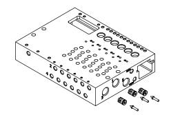
Diaphragm plug fixing
