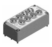
Power supply of the M8 analog outputs module is provided by 24VDC power input on the serial system (type A, 4 pin M12 power connector, pin 4) or by 5030.M12 additional power supply module, in case it were installed upstream of the outputs module. Modules provide M8 3 pins female connectors and a diagnostic LED for every analog input. The LED indicates signal presence (green) or overload fault (red).
