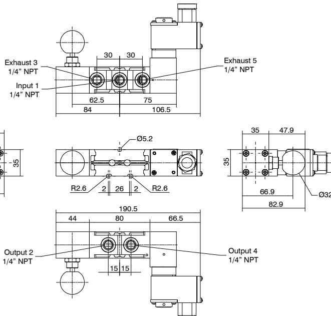
Minimum piloting pressure 2,5 bar
