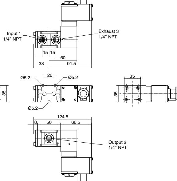
Minimum piloting pressure 2,5 bar
