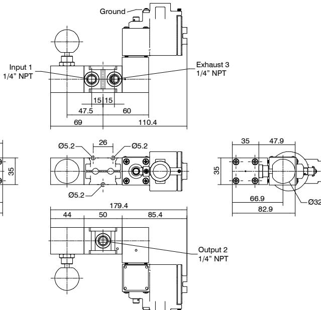
Minimum piloting pressure 2,5 bar
