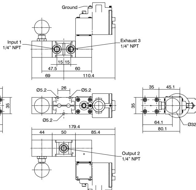
Minimum piloting pressure 2,5 bar
