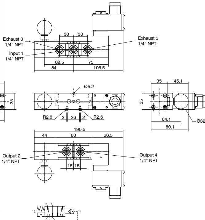
Minimum piloting pressure 2,5 bar
