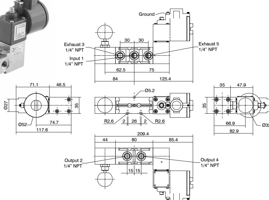
Minimum piloting pressure 2,5 bar
