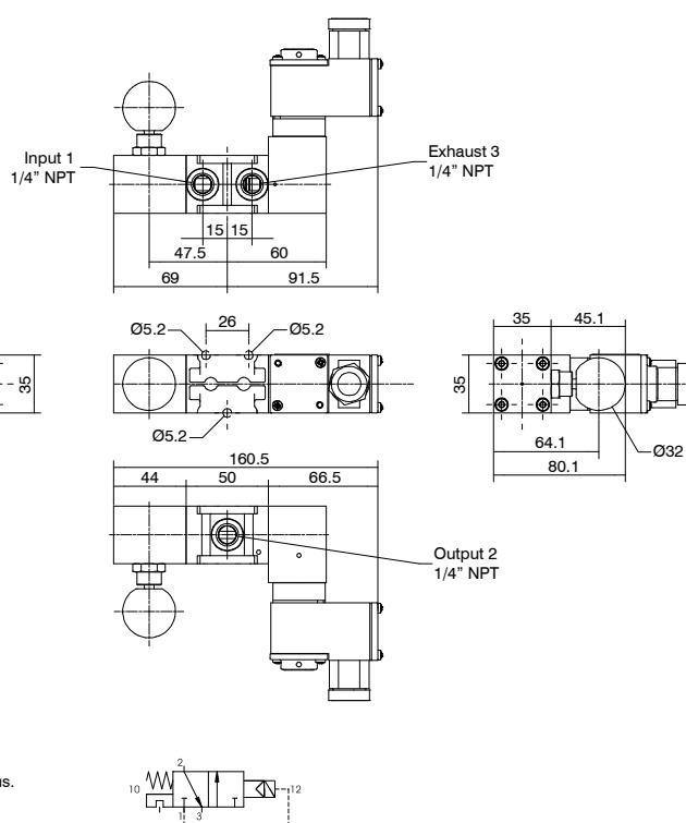
Minimum piloting pressure 2,5 bar
