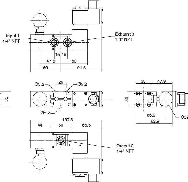
Minimum piloting pressure 2,5 bar
