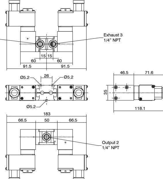
Minimum piloting pressure 2,5 bar
