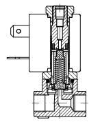
They can be **normally open (3/2 N.O.)** and in this case, at rest, the input orifice is open without electricity applied, the media reaches the intended use. Exhaust is closed.
