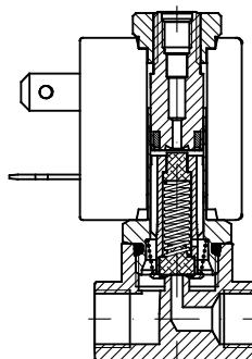
They can be **normally open (3/2 N.O.)** and in this case, at rest, the input orifice is open without electricity applied, the media reaches the intended use. Exhaust is closed.
