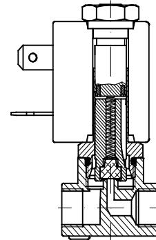
They can be **normally open (2/2 N.O.)**, in this case at rest the orifice remains open without electricity applied, the media reaches the intended use. When electricity is applied the input orifice closes.
