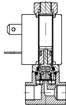
**Solenoid valves direct action 3-way:** 3-way solenoid valves have an input and an output connection in the valve body and an exhaust connection fitted in the stem of the core tube. The input and exhaust orifices are intercepted directly by the poppet fitted within the core tube.
