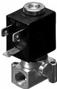
The bistable function is achieved by the use of a polarized permanent magnet energizing the coil with a DC current for at least 15ms in the reverse direction of the preceding impulse.
