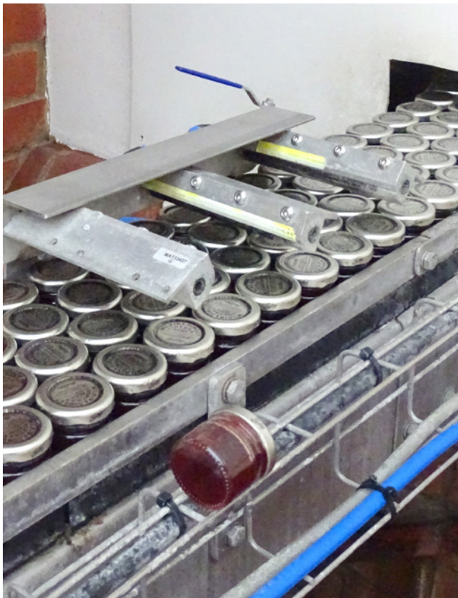
Air Curtains used to dry top of jars
