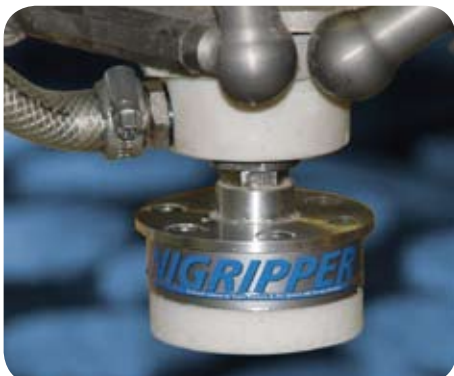
UniGripper for pick and place handling of biscuits.
