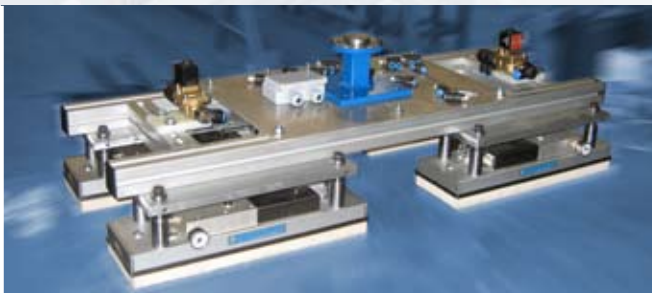
Special-tool with 4 SMS-grippers for bread-handling
