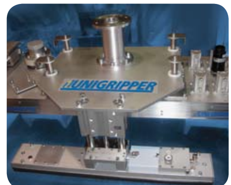
UniGripper with separate SMS-Gripper for the pallet handling.
