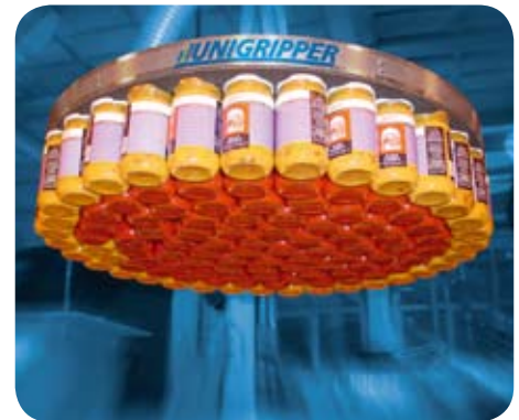
UniGripper for handling of different cans or jars into autoclave.
