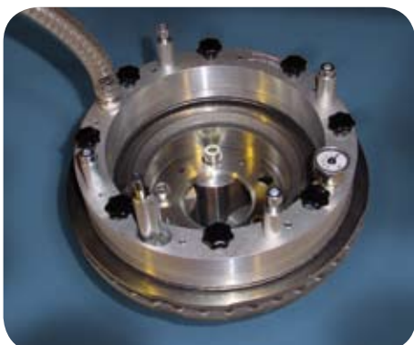
UniGripper customised for handling of brake discs in different shapes and sizes.
