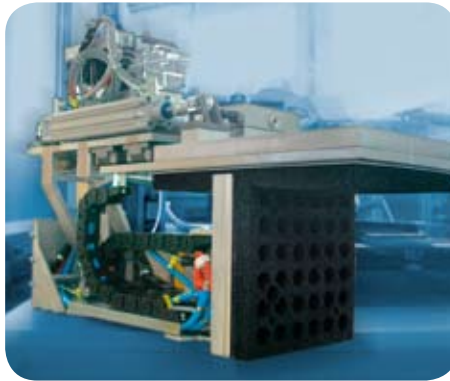
UniGripper custom built for automatic unloading of parcels from 40-foot containers.
