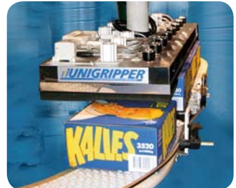
UniGripper Multichamber for optimized cycle-time and effective palletising.
