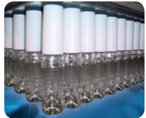
UniGripper BottleGripper for depalletising and palletising of PET- or glassbottles.
