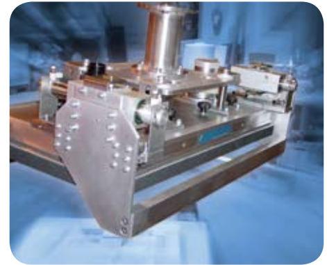
UniGripper equipped with side support for various layer/product sizes.
