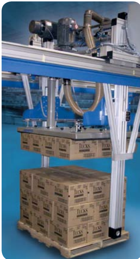
UniGripper LayerGripper handling full layers of heavy cardboard boxes in different sizes.
