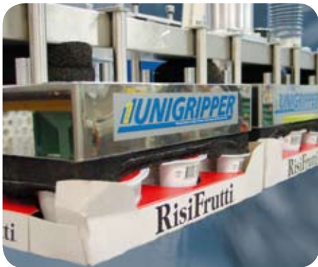
UniGripper handling of portion packs of food, packed in open trays.
