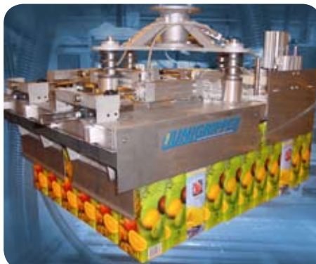
UniGripper for handling of single packages in different patterns.
