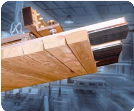
UniGripper for handling of different wooden products.
